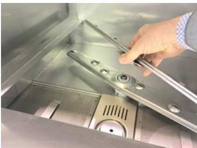
Remove the lower rinse arm
