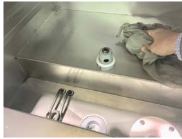
Wipe with a cloth the tank and check for any debris on the bottom.
