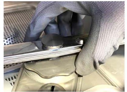
ATTENTION! Daily assemble the lower rinse arms by working on the „big“ ring nut, like in the picture.
