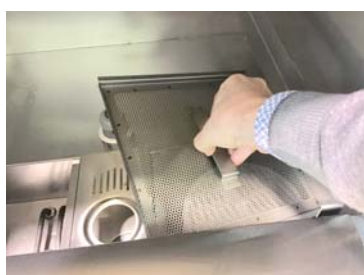
Remove the tank filters on the right
