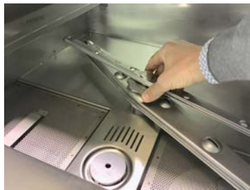
Unscrew the lower rinse arm
