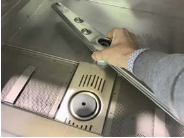
Replace the lower washing arm
