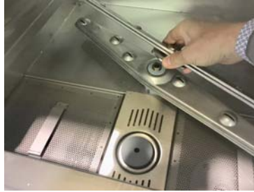
Replace the lower rinse arm
