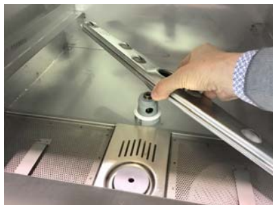
Remove the washing lower arm
