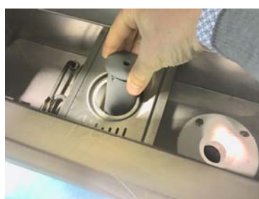
Insert the overflow
