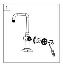
Step 1: Remove the handle button by hand. Loosen the screw with a Phillips screwdriver. Remove the handle and cartridge cap by hand.
