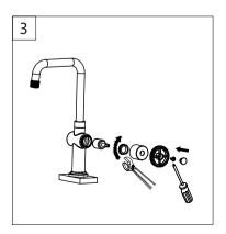
Step 3: Place the new cartridge in the handle seat. Secure the cartridge with the locking nut and assemble the handle.
