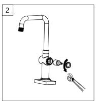
Step 2: Unscrew the locking nut with an adjustable wrench. Remove ceramic disc cartridge.
