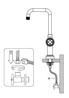
Connect hot and cold copper lines (4) to angle stops. Tighten both ends of waterlines with a wrench until snug. Turn on hot and cold angle stops and check for leaks.
