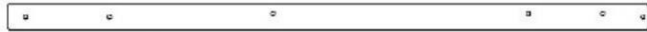
F1 | MONTANT MURAL - W4L12398 (x2) | 1 3/8 po x 2 3/8 po x 60 3/8 po (36 x 60 x 1 533)
