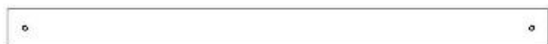
M6 | RAIL INFÉRIEUR - W4L12304 (x1) 5/8 po x 3 3/8 po x 47 po (16 x 86 x 1 194)
