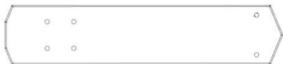
D01 PLANCHE DE RIVE DU PIGNON - W4L16415 (x8) 1 3/8 po x 5 1/4 po x 24 5/8 po (36x134x625)
