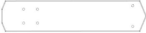
D01 PLANCHE DE RIVE DU PIGNON - W4L16415 (x1) 1 3/8 po x 5 1/4 po x 24 5/8 po (36x134x625)
