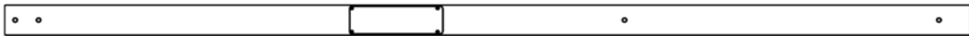
B2 | POTEAU - W2A03240 (1) | 72 mm x 72 mm x 2 305 mm (2 7/8 po x 2 7/8 po x 90 3/4 po)
