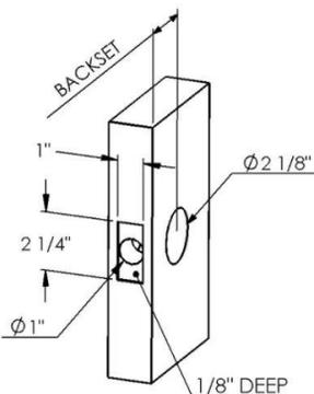
**Door Preparation:** The door prep is a set of drilled holes in the door, where the latch and levers will fit in.
