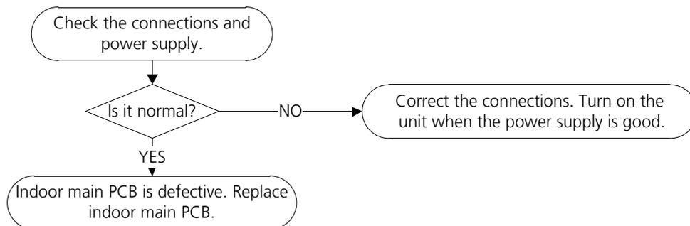
**Note:** EH 02 zero crossing detection error is only valid for the unit with AC fan motor, for other models, this error is invalid.
