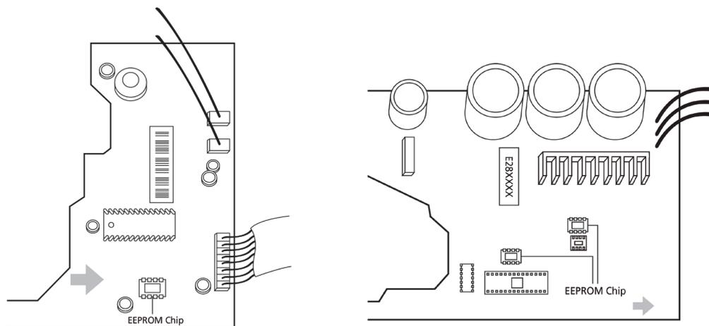
**Note:** For certain models, outdoor PCB could not be removed separately. In this case, the outdoor electric control box should be replaced as a whole. This pictures are only for reference, actual appearance may vary.
