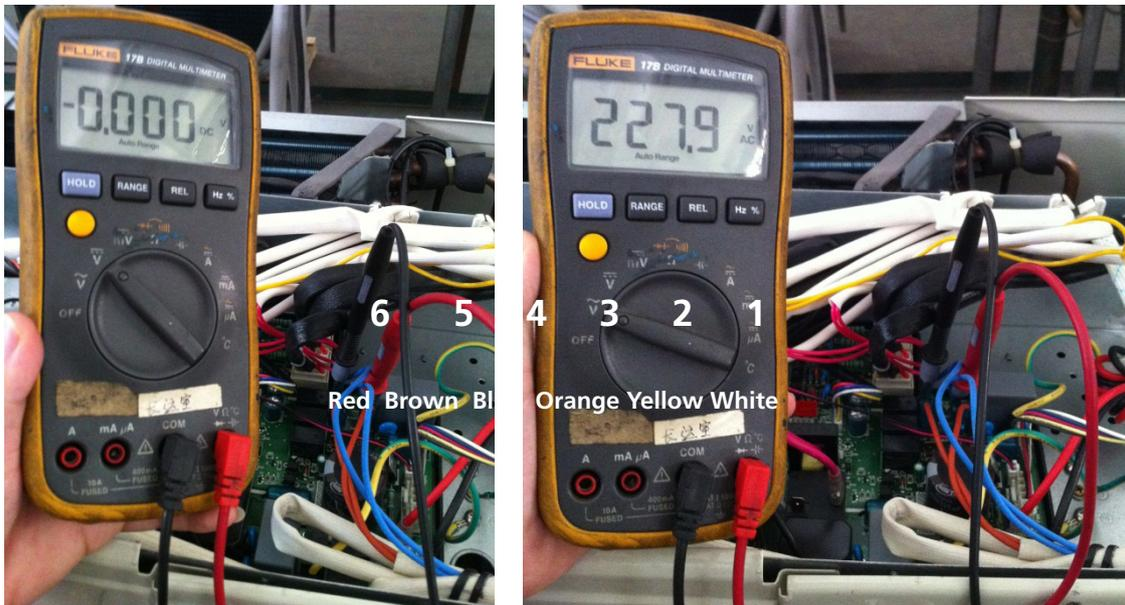
2 Turn off the power, use a digital tester to measure the resistance. The value should be 1.8~2.5 K $\Omega$ .
