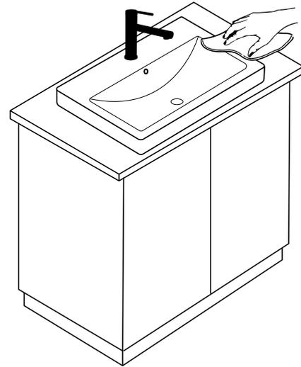
Push down on sink and ensure is stable and not rocking on countertop. Wipe away excess silicone caulk with damp cloth. Connect drain and water supply according to manufacturer's instruction.
