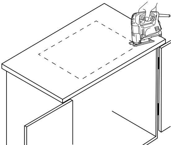
Trace the outline of the template and cut countertop according to templated outline using appropriate cutting tools. Template is for guide only. Use physical sink to ensure accurate cut-out opening.
