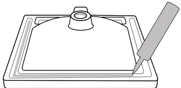
Clean sink flange and underside of cut-out area of countertop, making sure that the area is smooth and free of debris. Apply continuous bead of silicone.
