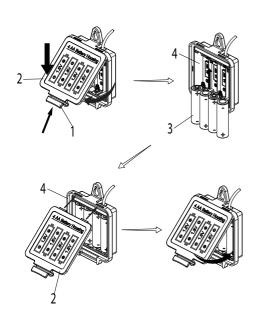
To open the battery housing, squeeze the tabs (1) on the cover (2), then remove the cover (2). Install the four AA batteries (3) included by matching the positive (+) and Negative (-) ends on the battery (3) to the (+) and (-) markings in the battery pack (4). The negative ends of the battery (3) should always connect to the spring end of the battery slots in the battery pack (4). Reinstall the battery pack cover (2) by pushing up and snapping into place.
