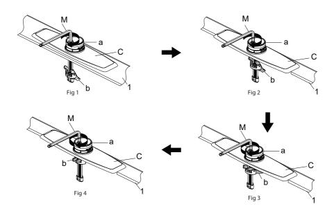
Press the base (a) and escutcheon (C) so that they can not move, then turn the screws with the provided hex wrench (M, HEX: 6.0mm) clockwise, as shown Fig 1. When the mounting plates (b) make contact with the sink (1), continue to turn the screw with the provided hex wrench (M, HEX: 6.0mm) clockwise, as shown Fig 2, until the base (a) is completely tightened and secured, as shown Fig.4.
