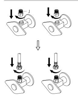
Before connecting waterlines to main valve, attach brass check valves (J) to angle stops (not included), then connect waterlines to brass check valves (J) and tighten until snug. Turn on angles stops and check for leaks (DO NOT TURN FAUCET ON)
