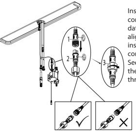
Install the data cable (1) to the control box connection (2). Ensure the arrows on the data cable and control box connection are aligned to one another to ensure proper installation. Ensure they are tightly connected by firmly pushing together. Secure the connection by hand tightening the nut (3) in a clockwise direction onto the threaded sensor cable.
