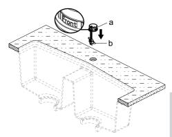
Shut off the water supply. Remove the old faucet. Clean the mounting surface. Check for the proper thickness of the sink. Insert the base (a) into sink. If your model does have a escutcheon, skip to step 1 b.
