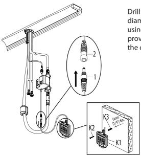
Drill a hole in the wall using a 6mm (1/4 in.) diamater drill bit. Install the battery pack (K1) using the molly anchor (K3) and screw (K2) provided. Insert the battery pack cable (1) into the control box connection (2).
