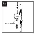
However, if you want to continue to use the faucet with the sensor feature, you need tight the switch button completely with a coin clockwise. At this time, you can use the faucet with the sensor feature.
