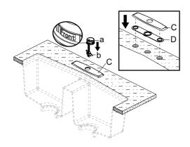
Place the escutcheon (C) and the gasket (D) on the sink. Insert the base (a) into escutcheon (C). Note: "Front" on the base (a) must face the front of the sink. The two mounting plates (b) on the base (a) must be loose and movable during the installation of the base (a). If the sink is uneven, use silicone under the gasket (D).
