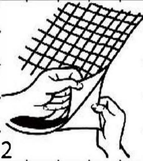
2. Peel off backing paper for a few centimeters.
