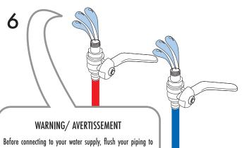
Betore connecting to your water supply, flush your piping to make sure it is free of sediment, flux, weld residue, deposits, debris or any other impurities that could damage your new faucet. Failure to rid your piping of the contaminants mentioned above will void your warranty and may result in premature failure, as well as property damage.
