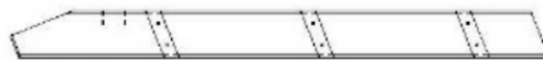
H79 MONTANT GAUCHE - W4L14944 (x1) 1 po x 3 3/8 po x 38 3/8 po (24 x 86 x 976)
