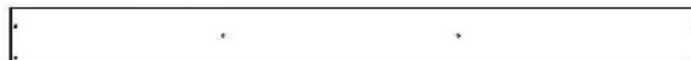
L2 PLANCHE DE PLANCHER - W4L14950 (x1) 5/8 po x 4 3/8 po x 54 3/8 po (16 x 112 x 1 382)
