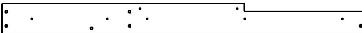
(1) K6 - LISSE MURALE CENTRALE AVANT - W4L11121 5/8 po x 5 1/4 po x 61 3/8 po (16x134x1560)
