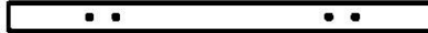
(1) O70 - PLANCHE DE MONTAGE DU TOBOGGAN - W4L09040 5/8 po x 1 3/8 po x 20 3/8 po (16x34x517)
