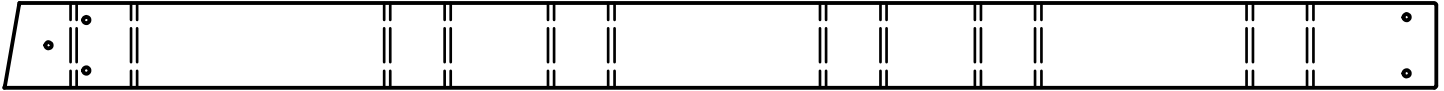
(1) A74 - HEAVY DUTY SWING BEAM EXT. WEB SWING - W4L11647 3 3/8"x5 1/4"x89 1/2" (86x134x2274)
