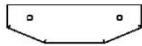
D05 | PLANCHE DE RIVE DU PIGNON - W4L16854 (x1) | 1 3/8" x 1 1/2" x 5 1/4" (36 x 38 x 134)
