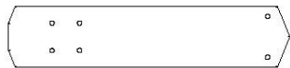
D01 | PLANCHE DE RIVE DU PIGNON - W4L16850 (x4) | 1 3/8 " x 5 1/4 " x 24 1/4 " (36 x 134 x 615)
