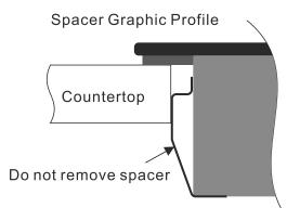
**NOTE**: The cooktops include spacers on both sides to ensure proper airflow once installed. Do not remove the spacers.
