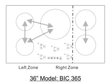
The power level displayed may be different from the actual power level at the power sharing and high temperature range. To prevent the cooktop from overheating, the power level is controlled automatically.
