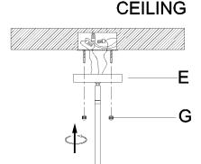
9. Install bulb (Not included) (Please do not exceed the maximum wattage recommended on the socket).
