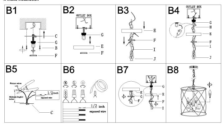
Step B1: Remove the collar ring (F) from collar loop (G). Attach the single bar (C) to outlet box with mounting screws (B). Besure that the side of single bar marked "GND" must face out, then unscrew the collar ring (F) from the collar loop (G). Step B2: Raise the canopy (E) through collar loop (G) and screw the collar loop (G) to measure a proper position.
