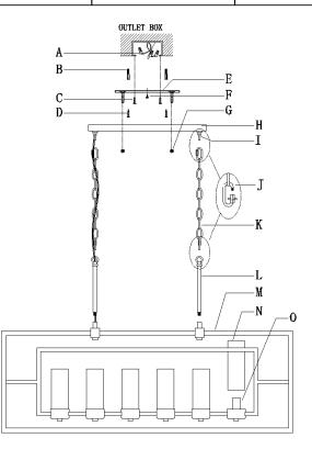
Step A1: Carefully pass the fixture wires through iron tubes (L), then screw iron tubes (L) onto iron frame (M).
