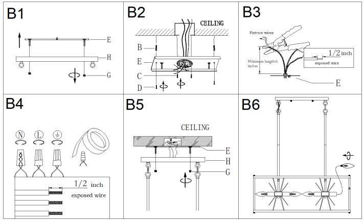
Step B1: Unscrew ball knobs (G) from mounting plate assembly (E) and gently remove canopy (H).
