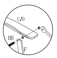
10. Attach the hinges (Part E) to the seat (Part B) with a screw (Part BB). Use 1 screw (Part BB) per side. The hinge can be affixed using either hole as the hinge is symmetrical.
