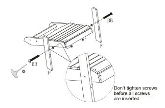
4. Run the screw (Part BB) through the seat (Part B). Secure the screw (Part BB) on the interior using the previously removed bolt. Do NOT tighten until all screws are inserted first.
