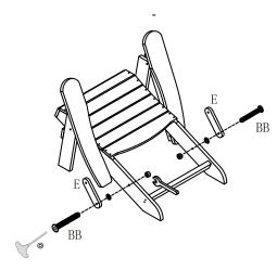
12. Secure the screw (Part BB) using the previously removed bolt.
