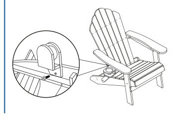
3. DO NOT TIGHTEN FULLY. It will allow you to angle and move the cupholder to the degree that you wish to set it.
