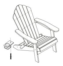
2. Run the screw with the washer (Part EE) through the cupholder and insert it into the underside of the armrest.
