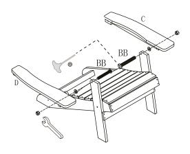
**8.** Attach the armrest (Part C or Part D) by running the screw (Part BB) with a washer through it.
