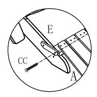
**16.** Align the holes of the armrest (Part C & D) with the holes of the backrest (Part A). Take 1 screw (Part DD) and remove the washer.
