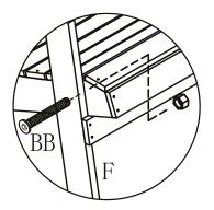
3. Run the screw (Part BB) ONLY through the front leg (Part F). Once that is done, attach the washer to the interior of the screw so that once installed, it will act as a buffer between the front leg (Part F) and the seat (Part B).
