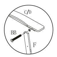
7. Run the screw (Part BB) through the front leg (Part F). Once that is done, attach the washer to the exterior side of the screw so that once installed, it will act as a buffer between the front leg (Part F) and the armrest (Part C or Part D).
