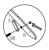
11. Run the screw (Part BB) through the seat (Part B). Once that is done, attach the washer to the interior side of the screw so that once installed, it will act as a buffer between the hinge (Part E) and the seat (Part B).
