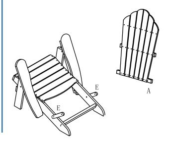
14. Take the backrest (Part A) and align it with the holes of the hinges (Part E). Remove the washer from the screw (Part CC).
