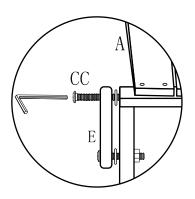
17. Run the screw (Part DD) through the armrest (Part C & D). Attach the washer on the interior of the screw (Part DD), so that it will act as a buffer between the armrest (Part C/D) and the backrest (Part A). Use an Allen wrench to tighten the screw. Repeat for the other side.
