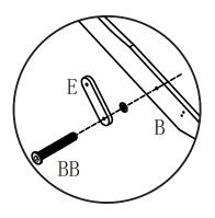
**13.** Angle the position of the hinges (Part E) to make it easier to attach the backrest (Part A).
