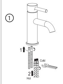
Preparation: Turn off water supplies and drain water lines. Clean installation site and remove any debris from the area.
