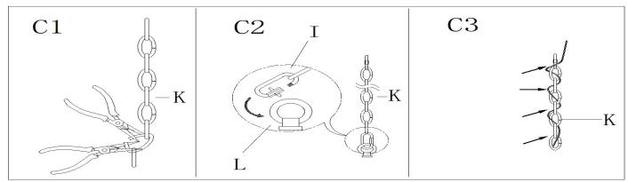
Step C1: By measuring, determine the correct number of links needed for proper hanging height. Using the chain pliers,
