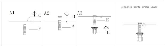
Step A1: Thread the single bar(C) over the nipple (E) a minimum of 6 mm (1/4"). At this point need note that: the side of single bar marked "GND" must face to the down.
