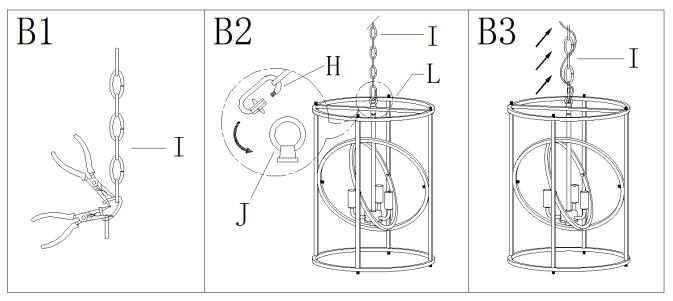
**Step B1:** By measuring, determine the correct number of links needed for proper hanging height. Using the chain pliers, disconnect and discard the unwanted part.
