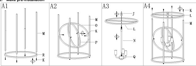
**Step A1:** Fix the tubes (M) to the lower iron ring (R) with screws (K).
