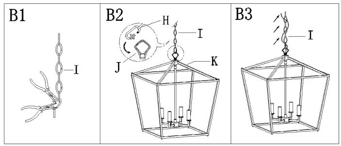
Step B1: By measuring, determine the correct number of links needed for a proper hanging height. Using the chain pliers, disconnect and discard the unwanted part.
