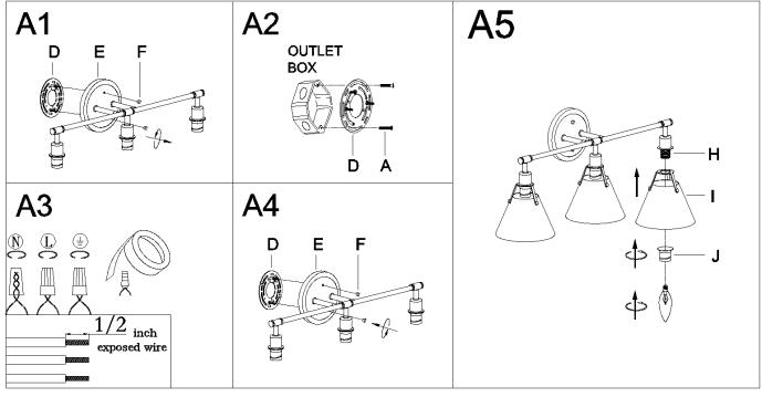
Step A1: Unscrew the ball knobs (F) from the back plate(E) then gently remove the mounting plate (D). Step A2: Secure mounting plate (D) to outlet box with mounting screws (A). Step A3: Make wire connections
