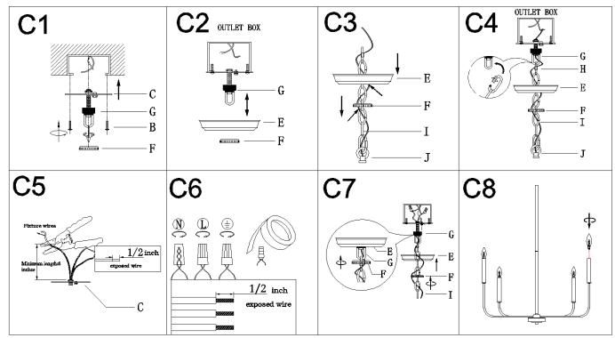
Step C1: Remove the threaded ring (F) from collar loop(G). Attach the single bar (C) to outlet box with mounting screws (B). The side of single bar marked "GND" must face out, Unscrew the collar ring (H) from the collar loop.
