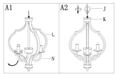
Step A1: Adjust connecting rods (L) and arms (N) to the proper position.
