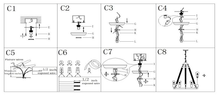
Step C1: .Attach the single bar (E) to outlet box with mounting screws (B). The side of single bar marked "GND" must face out
