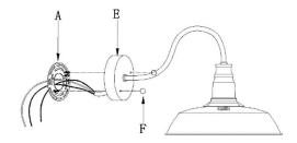
5. Attach the mounting plate assembly(A) to outlet box with mounting screws (C). Carefully and gently pass the outlet box wires through the mounting plate assembly(A).
