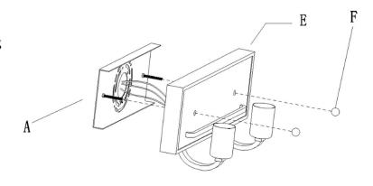
Step 2: Carefully pass wires from outlet box through back plate (A) Attach back plate (A) to outlet box with mounting screws (D)
