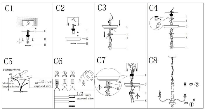
Step C1: .Attach the single bar (E) to outlet box with mounting screws (B). The side of single bar marked "GND" must face out Step C2: Raise the canopy (G) through screw collar loop (I) and screw the collar loop (I) to a proper position by measuring.
