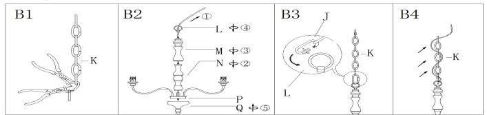
Step B1: By measuring, determine the correct number of links needed for proper hanging height. Using the chain pliers, disconnect and discard the remaining chain.
