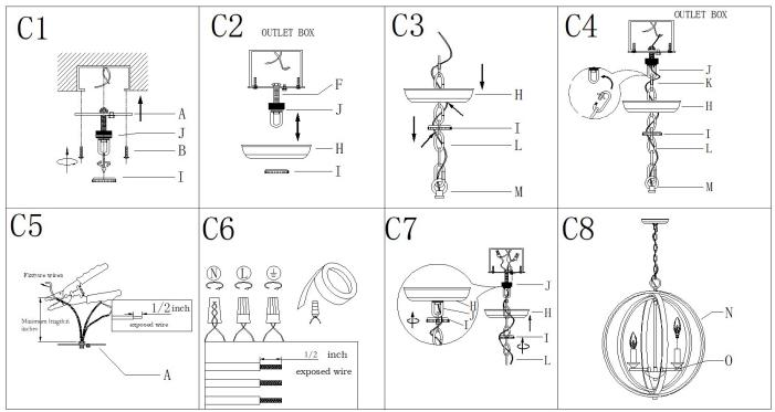
Step C1: Remove the threaded ring (I) from collar loop(J).
