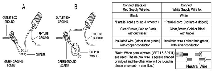
Twist plastic wire connector until wires are tightly joined together, wrap each connector with approved electrical tape. Be sure that no wire strands are exposed and carefully tuck all wires into the outlet box .
