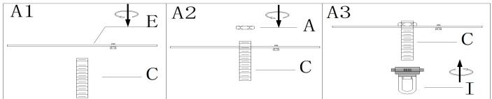
Step A1: Thread the single bar(E) over the nipple (C) a minimum of 6 mm (1/4"). At this point need note that: the side of
