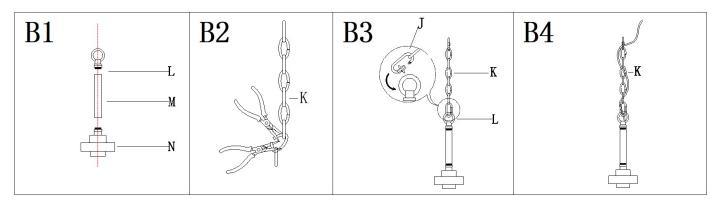
Step B1: Thread the tube (M)onto the top of lid till snug, and then thread the loop (L) onto the tube (M) till snug.
