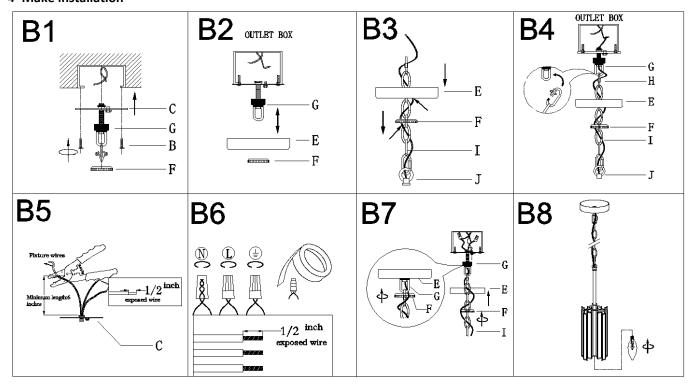
Step B1: Remove collar ring (F) from collar loop (G). Attach single bar (C) to the outlet box with mounting screws (B). Note: be sure that the side of single bar marked "GND" must face out.
