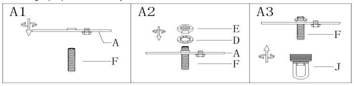
Step A1: Thread the single bar(A) onto the nipple (F), At this point need note that: the side of single bar marked "GND" must
