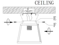
7. Fix the glass shade (I) onto the socket (G) with the socket ring (J). Install bulb (Not included) (Please do not exceed the maximum wattage recommended on the socket).
