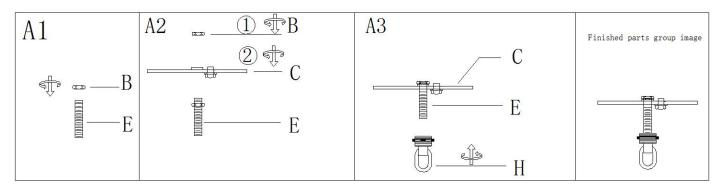
Step A1:Thread hex nut (B) onto the nipple (E)
