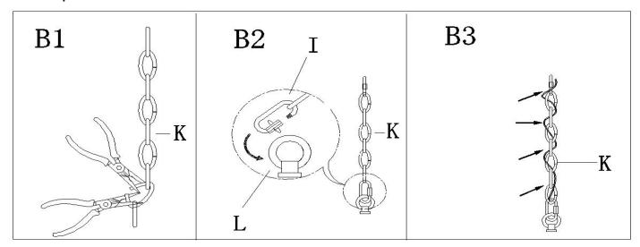
Step B1: By measuring, determine the correct number of links needed for proper hanging height. Using the chain pliers, disconnect and discard the remaining chain.
