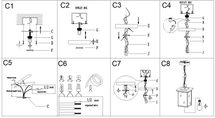
Step C1: Remove the collar ring (F) from collar loop (G). Attach the single bar (C) to outlet box with mounting screws (B). Note: be sure that the side of single bar marked "GND" must face out.
