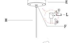
6. If needed, cut off the extra power cord length on the fixture 2 wires cord and green ground wire so that they all are at least 6 inches (152.4 mm) long within the outlet box
