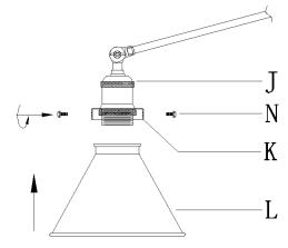
2) Carefully and gently pull the wires and fiberglass sleeve from the another end of arm(I) ,meanwhile push the socket (J) till two parts of joint are close each other , lay wires in the cave of joint(H), then proceed to push till the two parts are put together, secure with the stud
