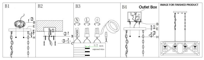
STEP B1: Unscrew the ball knobs (H) from canopy (E) then gently remove the mounting plate assembly (B)
