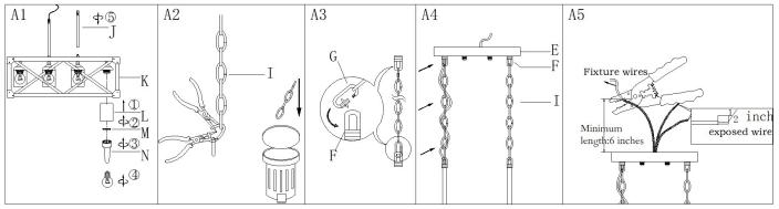
STEP A1:Place the glass shade (L)onto the socket of fixture (K)then use the spacer tool (N)to thread the socket ring (M) onto the socket to secure the glass shade in place.
