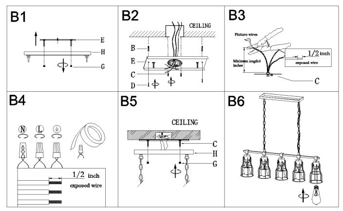
Step B1: Unscrew the ball knob (G) from mounting plate assembly (E) .
