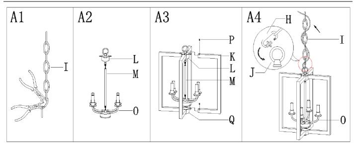
Step A1: By measuring, determine the correct number of links needed for proper hanging height. Using the chain pliers, disconnect and discard the remaining chain.
