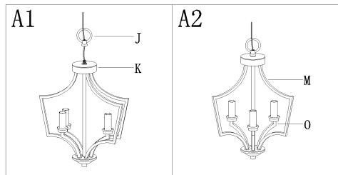
Step A1: Slip loop (J) over the wires and then thread it into the top of fixture loop (K).
