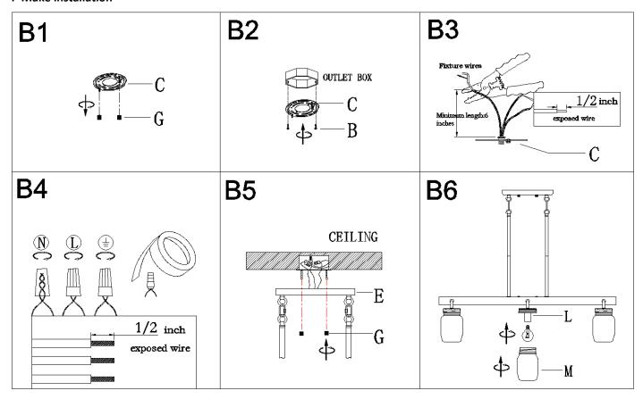
Step B1: Unscrew knob nuts (G) from round mounting plate (C).
