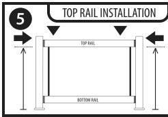
Fasten 2 balusters on BOTTOM RAIL to determine desired height of TOP RAIL. Position TOP RAIL with Connectors into place. Squeeze the top of posts slightly to leave impressions from gripping cones.
