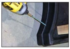
3. For the seat, using 4.5" screws, drill 1 screw into each section, through the wood. On the corners, make sure to drill on an angle. Do not overtighten.
