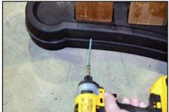
2. For the back rest, using 3.5" screws, drill 1 screw into each section, through the wood. Do not overtighten.
