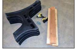
Tools Needed: Drill, 10 Deck Screws (3.5" L x 4, 4.5"L x 6), 5 pieces of lumber (up to 5' long).
