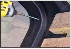
the slots. Make sure the wood is flush with the wood. On the corners, make sure to drill on an angle. Do not overtighten.
