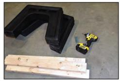
1. Tools Needed: Drill, 6 Deck Screws (3.5" L x 6), 5 pieces of lumber (up to 5' long).
